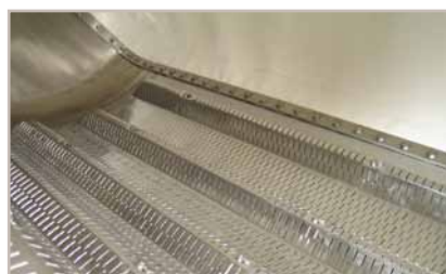
connected draining channels, electropolished
