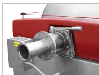
overfilling signalisation, axial filling valve
